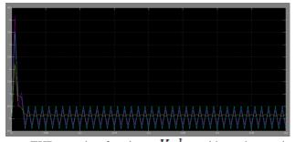
THD graph of voltage Vabc without harmonic correction(Y axis – THD, X axis - time in millisecond
