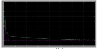
THD graph of voltage **Vabc** after harmonic correction(Y axis – THD, X axis – time in millisecond)
