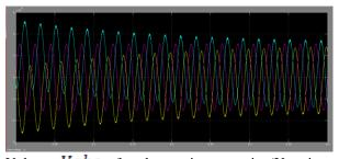
Voltage **Vabc** after harmonic correction(Y axis – Voltage in V, X axis - time in millisecond)
